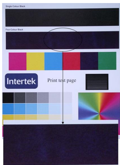
Close up of 4 colour black showing defect caused by too high a transfer current
